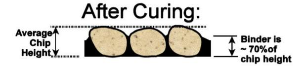
The figure above is a representation of before and after the curing process. Some cutback curing rates are faster than others. Such as Rapid curing cutback asphalt, which is used mainly for surface treatments and tack coat.
