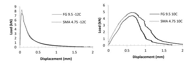
Figure 2 SCB load-displacement curve for mixes FG 9.5 and SMA 4.75: (Left) Load-CMOD curves at - 12°C, (Right) Load-LLD curves at 10°C.
