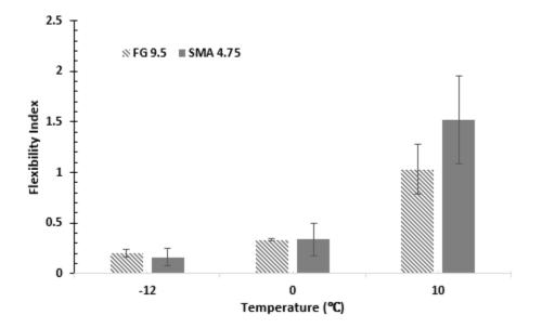
Figure 4 Flexibility index of FG 9.5 and SMA 4.75 at -12, 0, 10°C.
