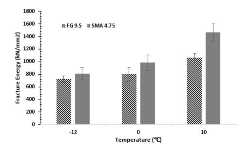
Figure 3 Fracture energy at -12, 0, 10°C for mixes FG 9.5 and SMA 4.75.
