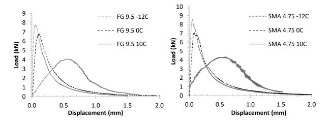
Figure 1 Load-displacement curves for mixes FG 9.5 and SMA 4.75 at -12, 0 and 10°C.
