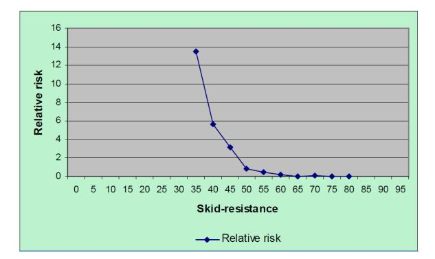
Figure 2 Relative rate of skidding-accident for different skid-resistance [13]
