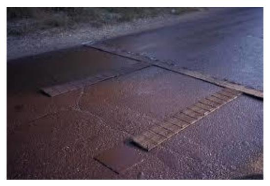
Figure 5. Weighing pads used to see how much tack coat has been applied [5]
