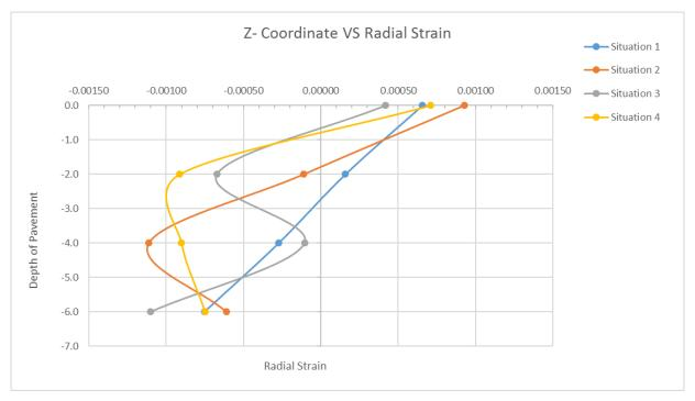
**Figure 3.** The relationship between the layers and the radial strains for the four different interface conditions.
