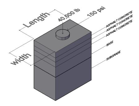
Figure 2. 3D geometry of the asphalt concrete pavement layer.
