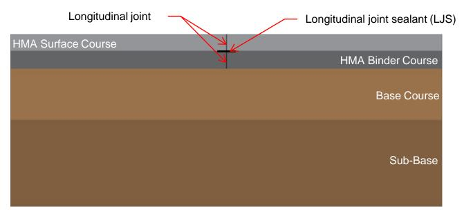
Figure 12. Section of roadway with LJS installed.
