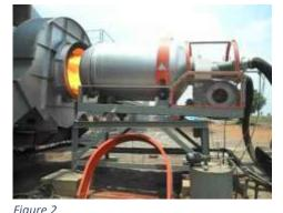
Burners remove the moisture content within the aggregate, and then the aggregate is heated to reach the needed temperatures. The safety hazards with burners are selfexplanatory. Letting the burner go unattended can cause problems. A common mistake that has been discovered is that many people are trying to adjust air or fuel mixture by feel instead of the gas analyzing, or even not keeping track
