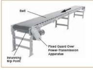
A conveyor system is a standard piece of mechanical handling equipment that moves materials from one location to another. Conveyors are especially useful in applications involving the transportation of heavy or bulky materials. The mechanical components include point of operation, power-transmission apparatuses, and other moving parts. The mechanical motions
