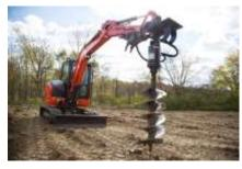
Augers are drilling devices that have a rotating screw blade referred to as a *Flighting* that is used to drill out material. Powered augers are mostly utilized in agriculture, landscaping, construction, and utility industries. They are commonly used to drill holes for pilings, utility poles, light poles, and fence posts. Many hazards come with an auger, whether it be with direct
