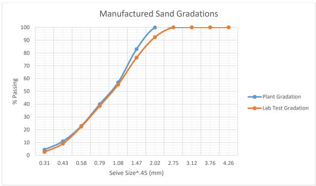
Figure 7: Manufactured Sand Gradations (Fine Aggregate)
