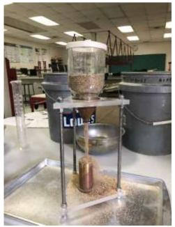
Figure 8: Uncompacted Voids Apparatus
