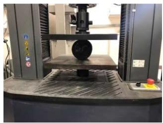
FIGURE 18a: Creep Test in Progress.
