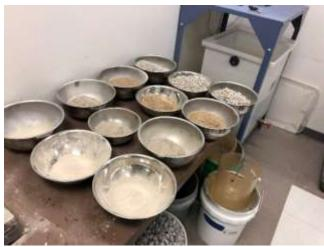
FIGURE 13: Aggregate Proportioning
