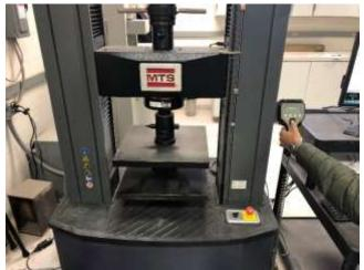
FIGURE 18c: Creep Test in Progress.
