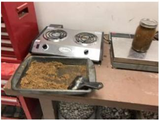
FIGURE 12: Fine Aggregate SSD Condition
