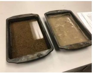
FIGURE 10: Fine Aggregate Water Bath
