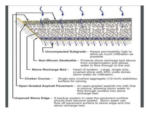
(National Pavement Association. "Cross-section of Porous Asphalt Pavement". *Innovative Stormwater Management Porous Asphalt Pavement with Subsurface Recharge Bed*. http://www.asphaltpavement.org /images/stories/porous\_asphalt\_ poster1.pdf.)
