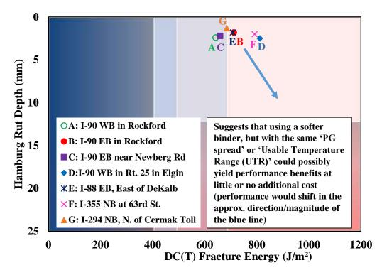
Figure 7. Performance-Space diagram of testing sections
