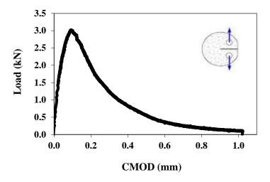
Figure 3. Typical Load-CMOD Plot
