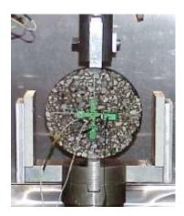
Figure 2. Indirect Tension Creep Compliance Test
