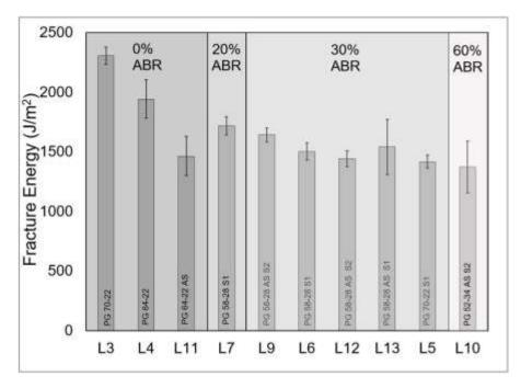
Figure 3 Intermediate-temperature (25°C [77°F]) SCB results for laboratory mixtures tested at a 50 mm/min (2 in/min) displacement rate.
