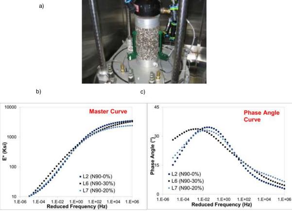
Figure 1 a) Complex Modulus Testing equipment, b) Modulus Master curves, c) Phase Angle Curve
