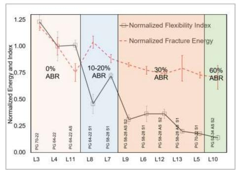
Figure 5 Normalized FI Results for the ICT Designed Plant Mixtures (FI Normalized based on mix L4)
