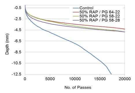
Figure 4.24. Average rut depths for District 5 mixtures with 50% RAP: effect of binder bumping.
