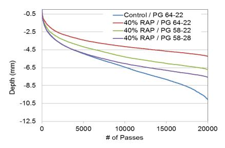
Figure 4.9. Average rut depths for District 1 mixtures with 40% RAP: effect of binder bumping.
