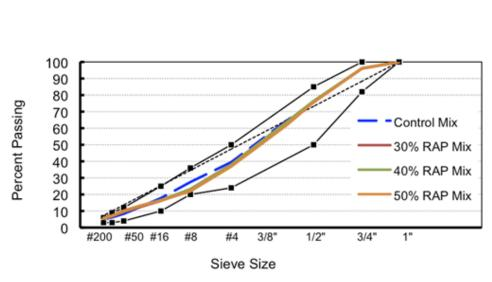
Figure 3.1. Aggregate blends for District 1 HMA designs.
