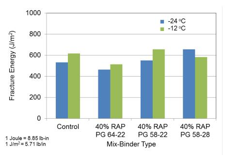
Figure 4.28. Fracture energies for District 5 mixtures with 40% RAP: effect of binder bumping.
