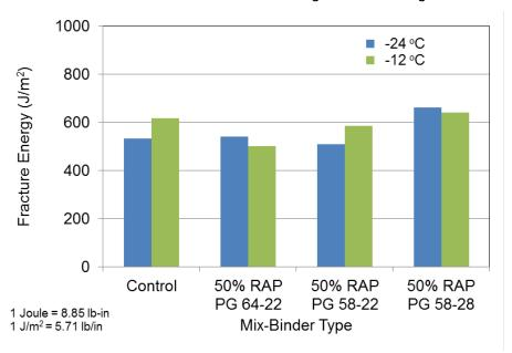
Figure 4.29. Fracture energies for District 5 mixtures with 50% RAP: effect of binder bumping.
