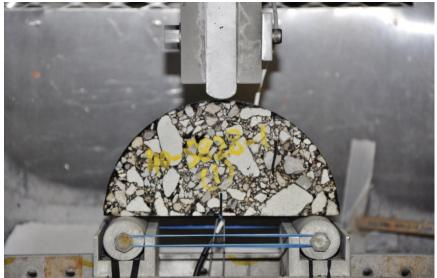
Figure 3.8. Semi-circular bending (SCB) test.
