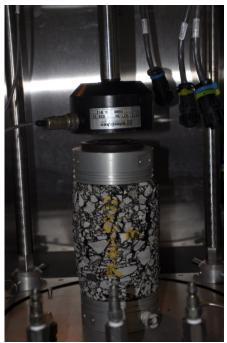
Figure 3.7. A specimen at the conclusion of a flow number test.
