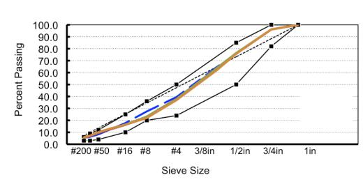
Figure 3.4. Aggregate blends for District 5 HMA designs.
