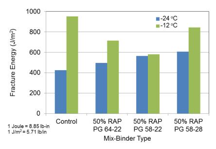
Figure 4.15. Fracture energy for District 1 mixtures with 50% RAP: effect of binder bumping.
