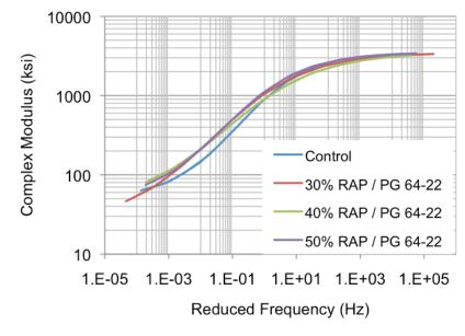
Figure 4.1. Master curves for District 1 control and HMA with RAP.
