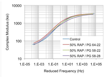
Figure 4.4. Effect of binder bumping on District 1 mixtures with 50% RAP.
