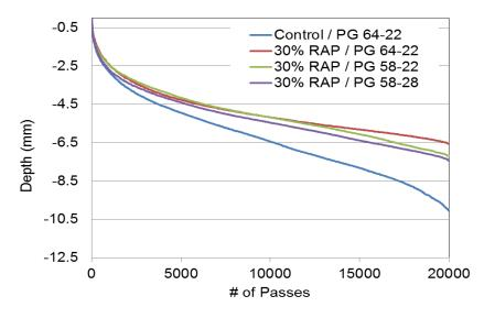
Figure 4.8. Average rut depths for District 1 mixtures with 30% RAP: effect of binder bumping.
