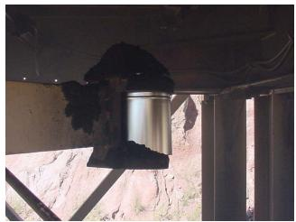
Figure 5. Mechanical tube sampling device.
