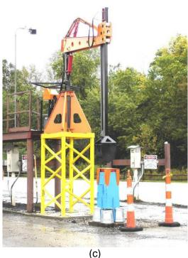
Figure 15. Mechanical sampling device experimented by Ohio DOT.
