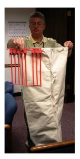
Figure 14. Sampling bag along with the sealed sample identification form.
