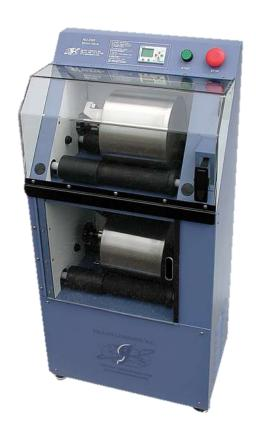
Micro-Deval tester used to evaluate coarse aggregates
