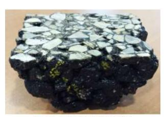
Fig. 6 - A chunk of bioasphalt
