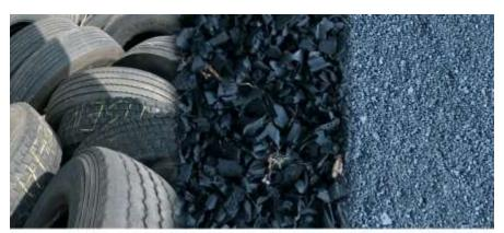
recycled granular materials are also mixed with unbound coarse aggregate and a type of polyurethane binder to form a porous pavement system
