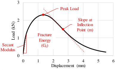
Fig. 1 Typical outcome from I-FIT test, after Ozer et al. [15]
