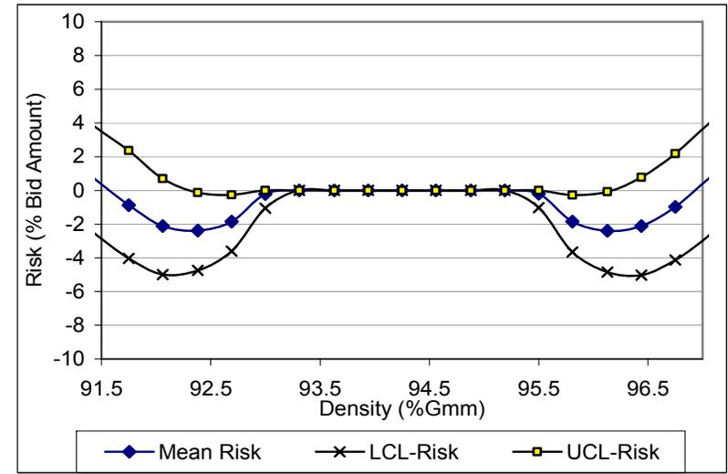
Figure. 3.9: Analysis results for low production variability and medium number of specimens: old vs. new PF equation
