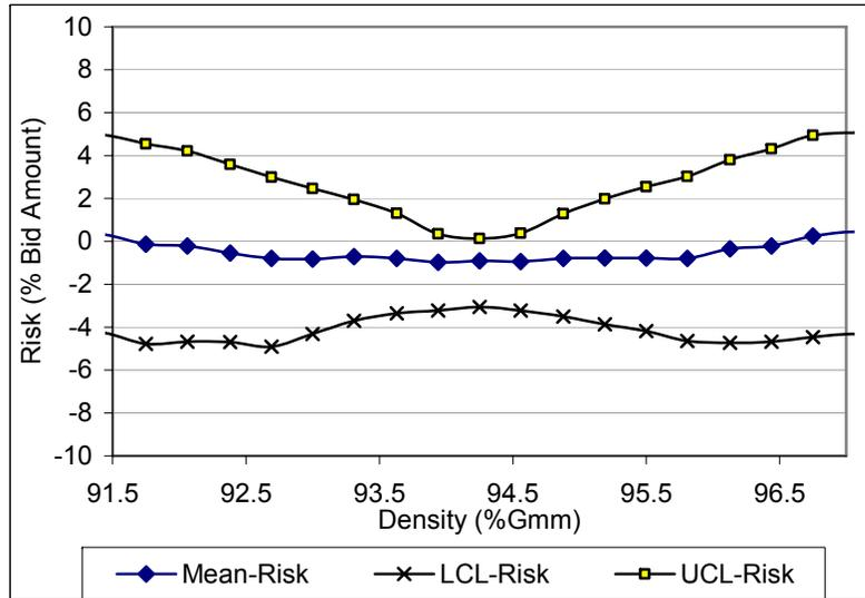
Figure. 3.8: Analysis results for high production variability and low number of specimens: old vs. new PF equation
