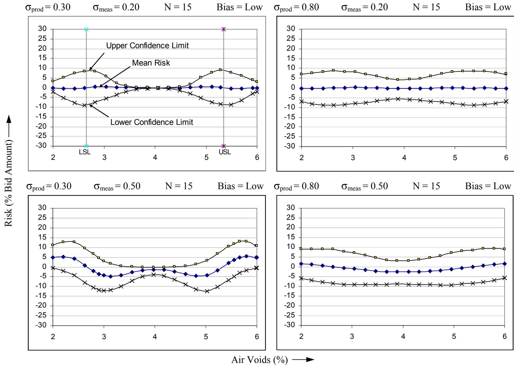
Figure 3.1: Sensitivity analysis simulation run plots from SRA (LSL, USL: Lower and Upper Specification Limits)
