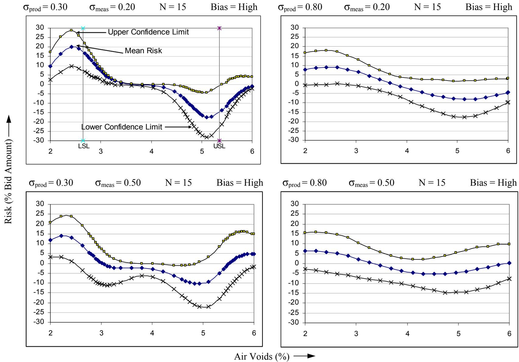
Figure 3.2: Sensitivity analysis simulation run plots from SRA (LSL, USL: Lower and Upper Specification Limits)
