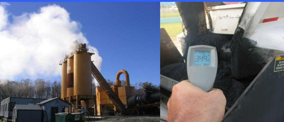
Research by Stroup-Gardiner and Lange at AU Indicates increased emissions with increased temp. We Can Reduce Temperatures Today with No Additives
