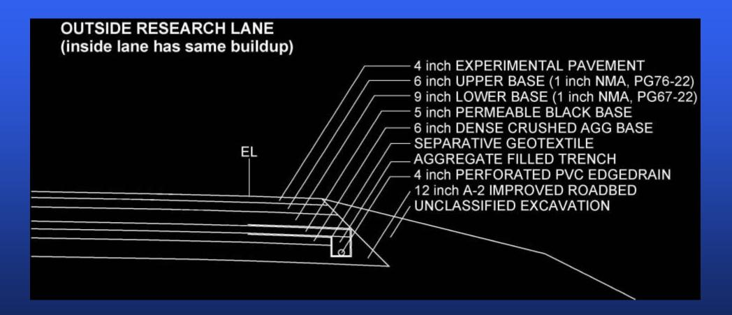
21" HMA, 5" AC Treated Drainable Base, 6" Aggregate
