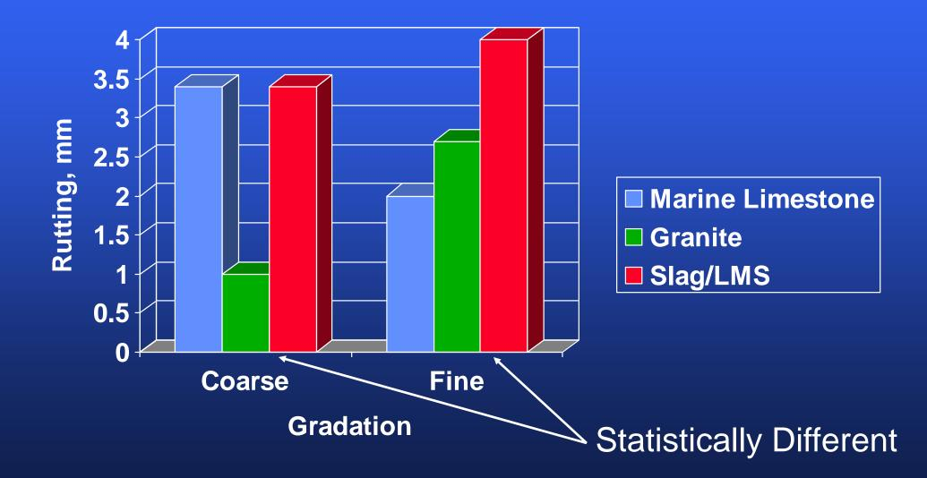
Fine graded and coarse graded mixes perform approximately the same in rutting
