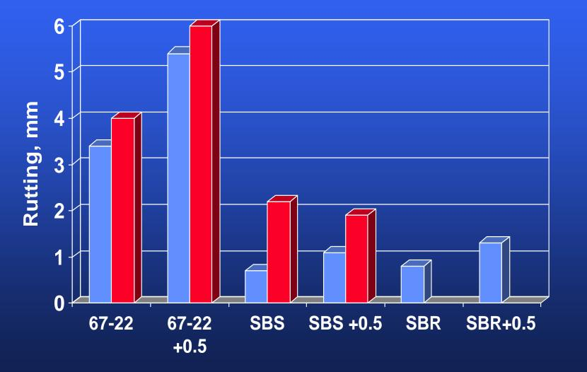
BRZ ARZ Modified mixes (PG-76) rutted 66% less than unmodified (PG-67) mixes
